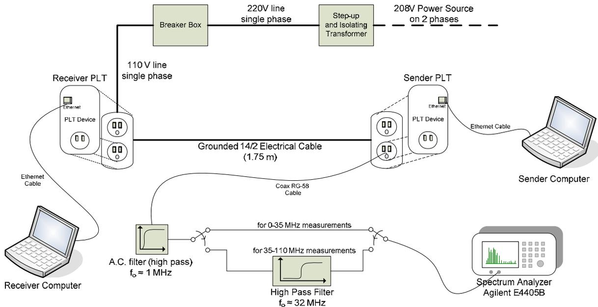
The conducted power measurements were made over the frequency range from 0 to 110 MHz using two modes of operation: Data Transfer mode and Idle mode (no active data transfer). The goal of the tests was to determine the output level injected into electrical lines up to 110 MHz in both modes and the bandwidth and spectral shape of the PLT devices.
