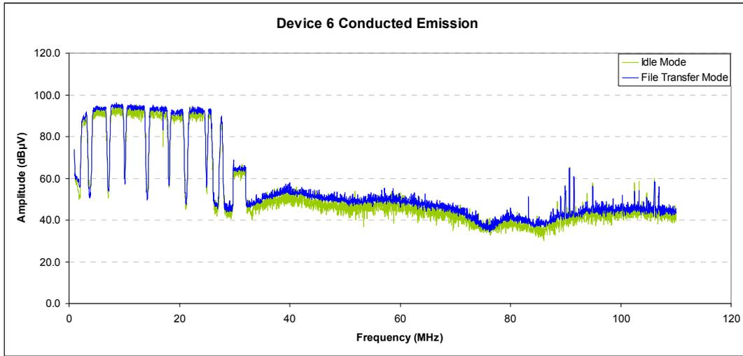
These results illustrate that the potential for interference is pervasive and continuous from a PLT device. Even if the PLT device is not transmitting data, the device is actively generating emissions. It is also observed that even if the PLT device operates below 30 MHz, the device significantly raises the noise floor up to at least 80 MHz.
